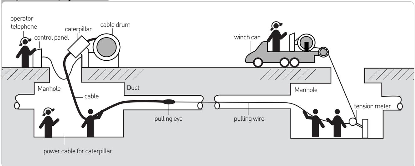
Fig. 5 Cable Laying at Tunnel
