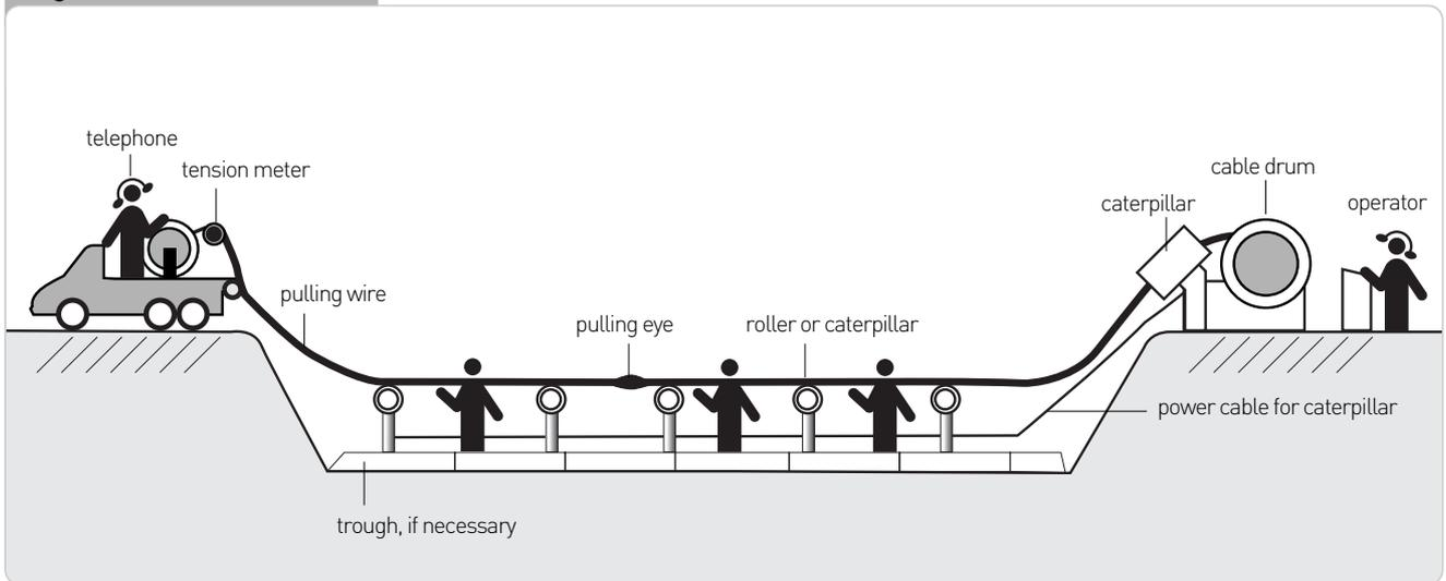
Fig. 4 Cable Laying at Duct
