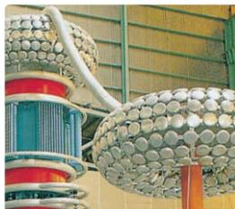
\*High Voltage Test Transformer
