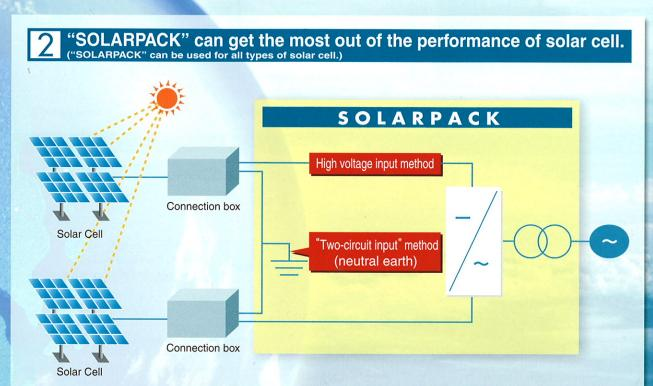
Two-circuit input method is suitable for thin-film solar cell, because, owing to the wide range of input voltage, it can make the best use of generated output, even if solar cell has wide range of voltage fluctuation such as thin-film solar cell.
